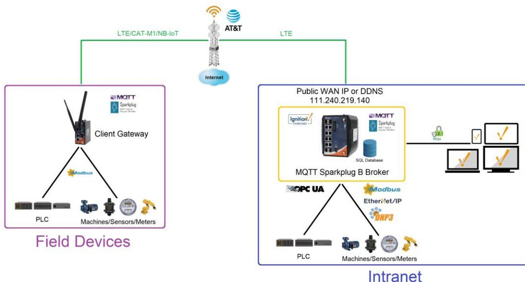
Ignition MQTT Broker installed onboard in IGMG-P83244GC+-D4G Gateway makes the system self-contained and more cost effective when a Cloud server does not have to be used. End-devices can access the MQTT server remotely and directly with its Public WAN IP or DDNS address. Ignition running in user's premises can work with local clients and devices and simultaneously provide a possibility of data visualization and storage as well as end-devices control via cellular link.
