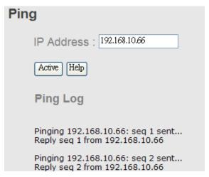
After you press **Active**, four ICMP packets will be transmitted, and the sequence number and roundtrip time will be displayed upon reception of a reply. The page refreshes automatically until responses to all packets are received, or until a timeout occurs.
