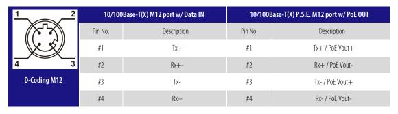
Note: pins 1 and 3 (-Vdc) should not be shorted to ground.
